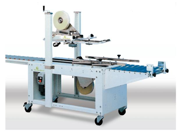
This hand fed case taper is suitable for short or long runs of the same case size and can seal cases from 50mm high with self-adhesive tape.
