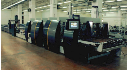
Folder gluers up to 2.3 m from Duran Machinery, Turkey
