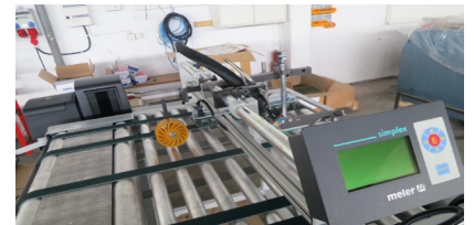
Semi automatic hot melt gluers from Arapak
