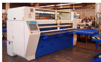
Boxmaker for Corrugated from Bizzozero, Italy
